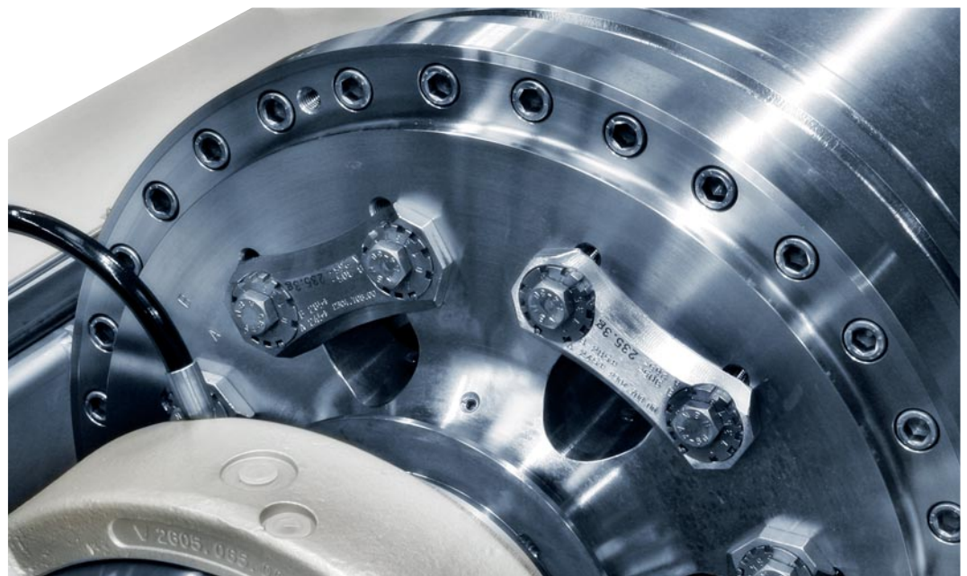
The picture shows a decanter rotor with eccentric adjustable weir plates.
