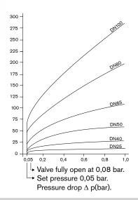
This diagram shows the flow characteristics depending on the pressure drop
