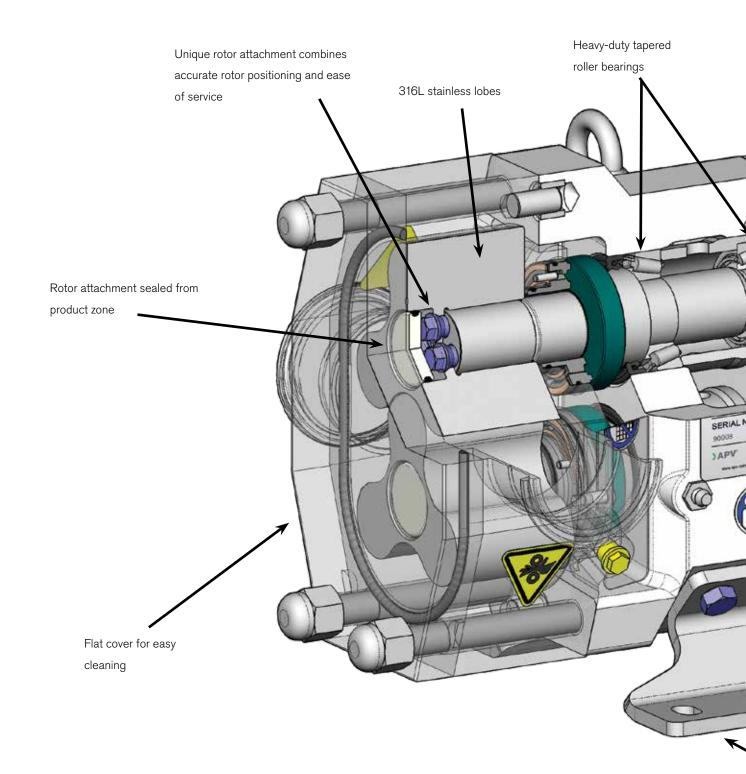
Easy access to shims for rotor clearance adjustment
