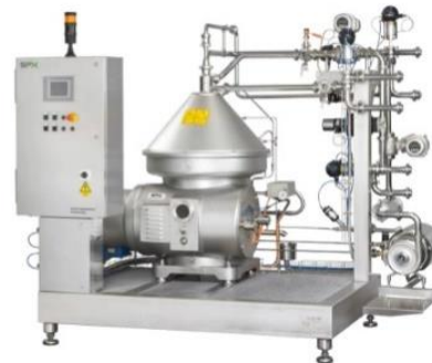
Combination of accessories and separators in skidded solutions
