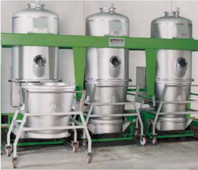
Batch fluid beds with removable product containers
