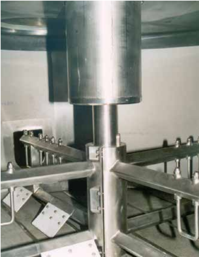
Inside view of an Anhydro fluid bed with an agitator in the product inlet section
