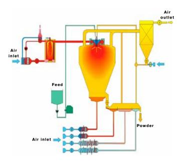
The fines are conveyed with the drying air to the wet zone in the drying chamber top, where the fines agglomerate with the wet droplets. Fines carried out together with the air are separated from the air in a cyclone system or a bag filter, and the fines are re-circulated to the atomizer zone for agglomeration.
