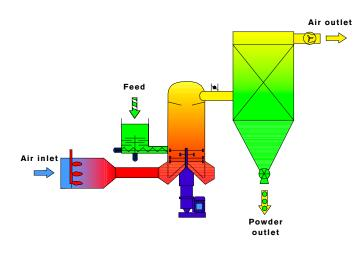
The feed material is screw-fed to the compact drying chamber and disintegrated by the agitator at the bottom of the chamber. The product is fluidized by the hot air entering tangentially. The dried powder leaves the chamber at the top through a classifier and is separated from the drying air and discharged from a bag filter.
